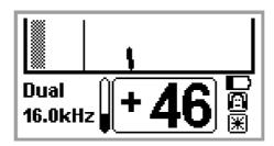
When the graph is clearly bent, curved or spread across the whole of the display, it is highly probable that you are dealing with an object such as a can, a thin steel sheet or other steel object whose magnetic properties are lesser than its conductive properties.
