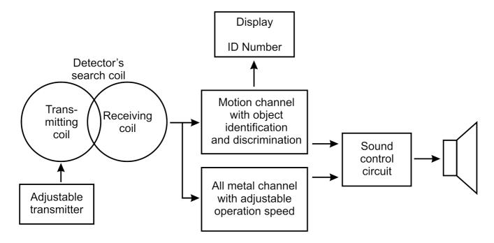
Argo NE consists of several basic functional blocks: a transmitter, a search coil, a Motion channel, an All metal channel, a sound control circuit and parts used to communicate with a user: a display and a speaker.
