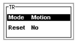
The buttons are used to select the operating mode you would like, then press the trigger to enter the program. After changing the operating mode a ground balance needs to be done, and the detector will guide you through this process.
