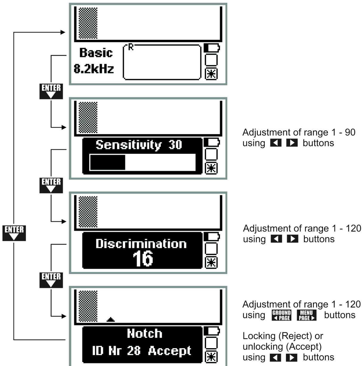
After pressing the **ENTER** button the « Sensitivity » message will appear on the display, a number describing the Sensitivity level and a linear scale showing the adjustment range. The adjustment is done using the **◀ ▶** buttons. Pushing the **ENTER** button a second time will show the Discrimination level. Adjusting the Discrimination is done in the same way as adjusting the Sensitivity.
