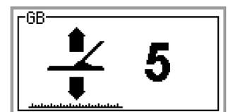
Most soil types gives a phase reading of around -87.0. Wetlands can produce higher phase readings (e.g. -83.0). Should the ground balance results be noticeably higher than these values (e.g. -75.0), there is a high probability that some metal objects are present in the balance area. The ground balance should be repeated again at a different location a few metres away.
