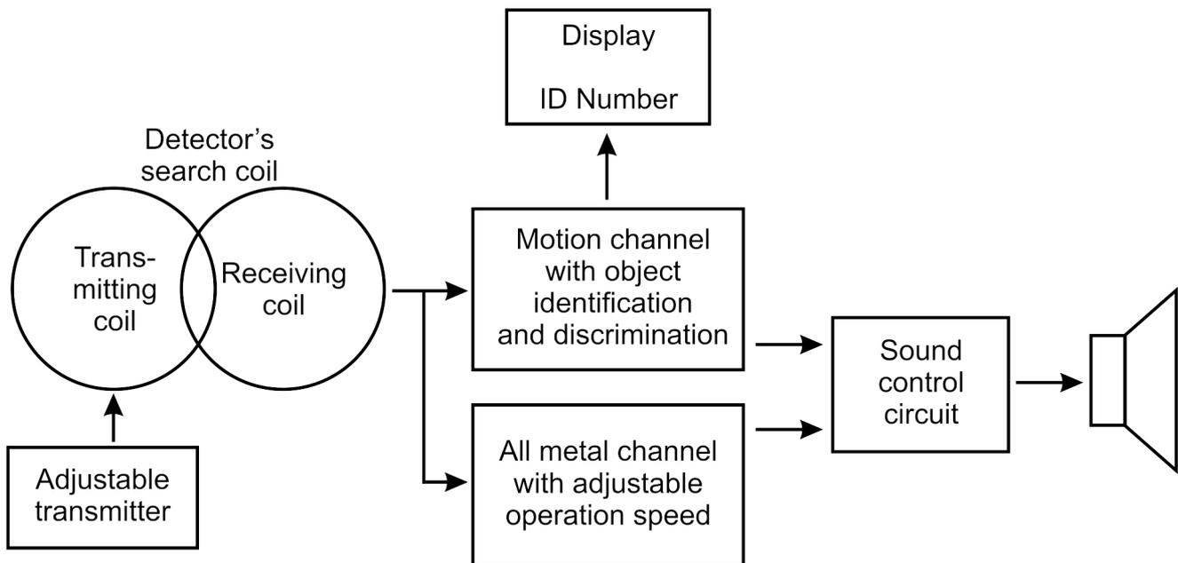
Alter71 consists of several basic functional blocks: a transmitter, a search coil, a Motion Channel, an All metal channel, a sound control circuit and parts used to communicate with a user: a display and a speaker.
