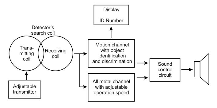
Ultima consists of several basic functional blocks: a transmitter, a search coil, a Motion channel, an All metal channel, a sound control circuit and parts used to communicate with a user: a display and a speaker.
