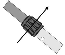
NOTE: Try to avoid creating large loops of cable near the edges of the search coil, as this may result in the detector giving false readings.
