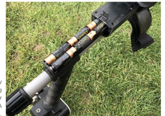
Battery housing for six AA batteries.
