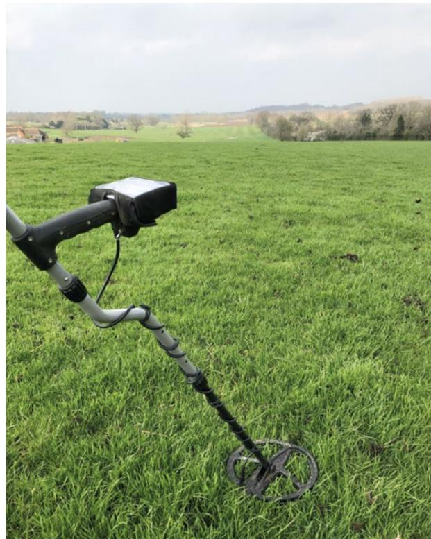
**Dual Mode** This combines the all metal channel with the motion discrimination channel. Once I got used to the machine, I found this mode to be the most informative.
