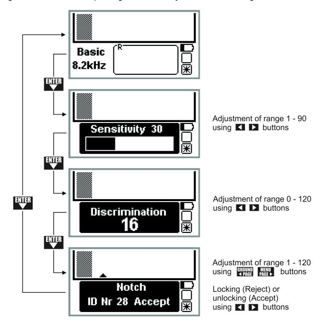
After pressing the button the « Sensitivity » message will appear on the display, a number describing the Sensitivity level and a linear scale showing the adjustment range. The adjustment is done using the buttons. Pushing the button a second time will show the Discrimination level. Adjusting the Discrimination is done in the same way as adjusting the Sensitivity.
