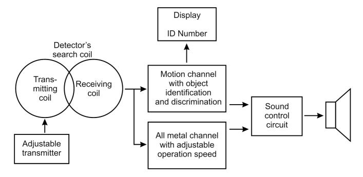
Alter71 consists of several basic functional blocks: a transmitter, a search coil, a Motion Channel, an All metal channel, a sound control circuit and parts used to communicate with a user: a display and a speaker.
