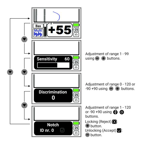
After pressing the volume button the « Sensitivity » message will appear on the display, a number describing the Sensitivity level and a linear scale showing the adjustment range. The adjustment is done using the volume buttons. Pushing the volume button a second time will show the Discrimination level. Adjusting the Discrimination is done in the same way as adjusting the Sensitivity.
