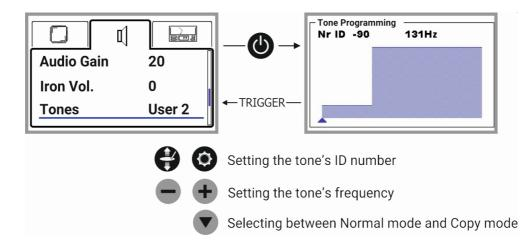
After selecting a suitable sound profile from the User group it can be edited by pressing the button. The buttons are used to choose the ID number for which a specific tone is applied, to change the frequency of the sound are used the buttons. The ID number currently edited is shown by a digit and a cursor (a red triangle for the Copy mode and a blue one for the Normal mode) which are shown at the bottom of the display.
