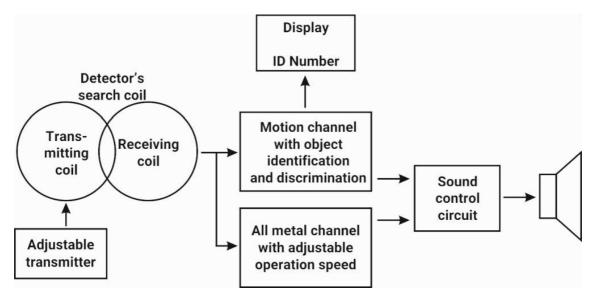
Atrex consists of several basic functional blocks: a transmitter, a search coil, a Motion Channel, an All metal channel, a sound control circuit and parts used to communicate with a user: a display and a speaker.
